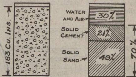
FIG. 3—TYPICAL CALCULATION FOR ABSOLUTE DENSITY OF A MORTAR (MORTAR 1:2)
