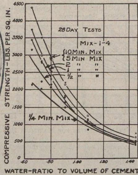
FIG. 7—INFLUENCE OF WATER ON THE STRENGTH OF CONCRETE Water-strength curves for each time of mixing. Each value is the average of 4 tests from the same batch. Water content calculated as a ratio of the volume of cement. From paper by Prof. D. A. Abrams previously published in The Canadian Engineer.
