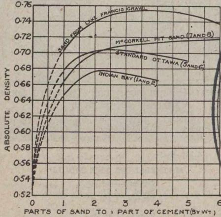
FIG. 5—COMPARISON OF ABSOLUTE DENSITIES OF MORTARS FROM SANDS OF DIFFERENT GRADING
