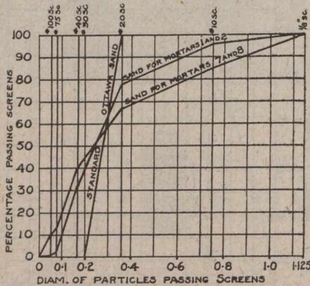
FIG. 6—MECHANICAL ANALYSIS DIAGRAM FOR SANDS USED IN TESTING AFFECTS OF ALKALI SOLUTIONS UPON VARIOUS MORTARS
