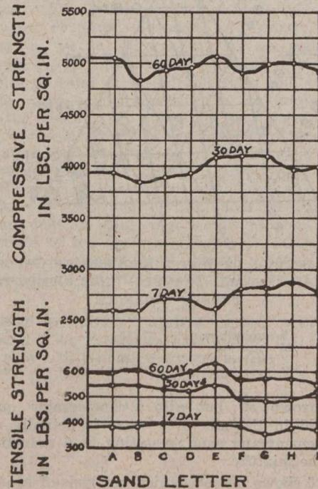
FIG. 8—STRENGTH TEST OF MORTARS OF SAME CEMENT-SURFACE AREA RATIO BUT DIFFERENT VOLUMETRIC PROPORTIONS—FROM PAPER BY CAPT. L. N. EDWARDS
