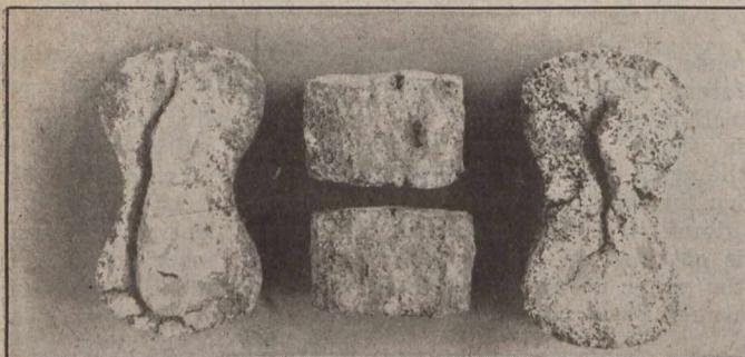
ACTION OF A 10% SOLUTION OF MAGNESIUM SULPHATE ON No. 14 MORTAR
