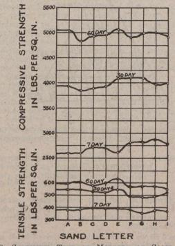
FIG. 8-STRENGTH TEST OF MORTARS OF SAME CEMENT-SURFACE AREA RATIO BUT DIFFERENT VOLUMETRIC PROPORTIONS-FROM PAPER BY CAPT. L. N. EDWARDS
