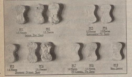
ACTION OF A 10% SOLUTION OF MAGNESIUM SULPHATE ON VARIOUS MORTARS
