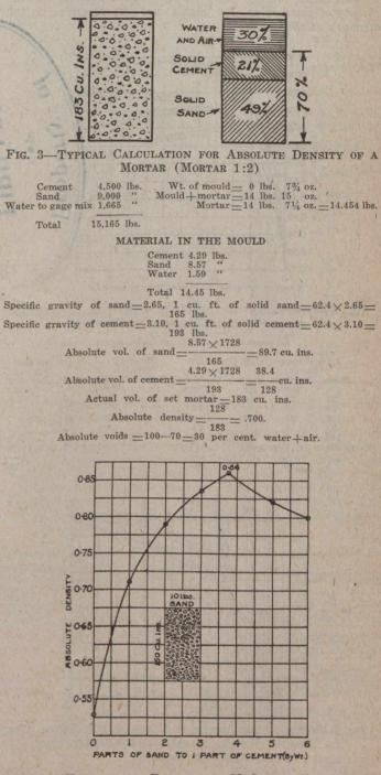
FIG. 4-THEORETICAL DENSITY OF MCCORKEL PIT SAND MORTARS
