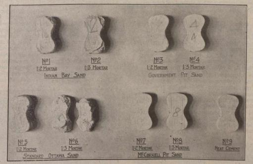
ACTION OF A 10% SOLUTION OF SODIUM SULPHATE ON VARIOUS MORTARS Air briquettes cured 24 hrs. in moist closet and 48 hrs. in steam at 150 degs. F. kept in alkali solution for 3½ months. No. 1 shows slight action at edges; No. 2, disintegration at ends; Nos. 3,4 and 5, no apparent action; No. 6, disintegrated; Nos. 7, 8 and 9, no apparent action.
