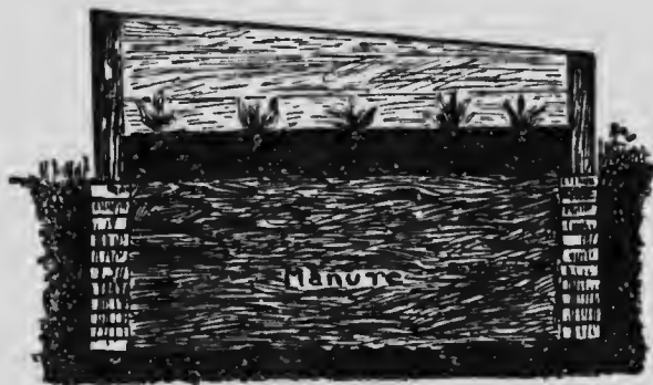
Sectional view of a hotbed
