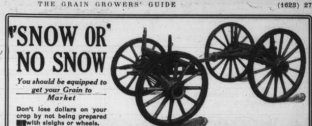
G.G.G. Canadian Farm Trucks are easy running and made to stand the wear and lear of heavy work on Western Farms. A patented groove collar skein makes the bearing sand proof. Skeins are long and go well up on the axle giving added strength. Full clipped gears are made of air-seasoned hard wood; axles are hickory and hounds white oak. Bolsters are well ironed and have 14 inch stakes, well braced and hinged. The wheels have se-lected oak in hubs and rims.
