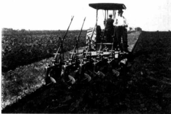
A 16-32 Kerosene burning Tractor pulling a 5 bottom 14-inch Cockshutt Engine Plow
