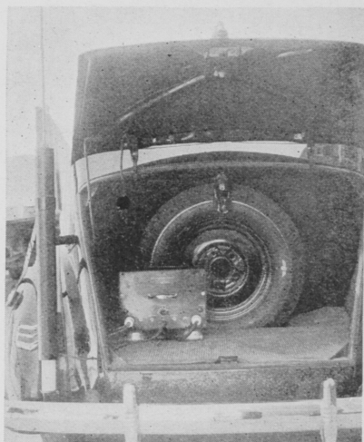
View of transmitter installed in car trunk.
