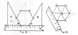
to that shown by the dotted lines and draw fe. Reverse the square and draw cd. Make each of these two inches. Join ed. A good variation of this exercise, and one that requires care, is to draw the hexagon without measuring anything but the base (Fig. 20). Draw ab the required length. Draw af and bc as before, but without measuring. After drawing af, slide the square to b and draw bc. Similarly from the position at bc slide the square to a and draw ad.
