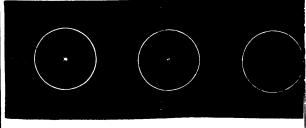
FIG. 39.—Fizeau's velocity of light apparatus. Appearance when the toothed wheel is at rest, when it is in slow motion, and when its rotation is so rapid as to cause complete extinction of the light.
