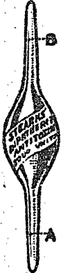
SEALED ANTITOXIN - BULB - SNAP NECK AT A AND ATTACH NEEDLE SNAP AT D AND ATTACH RUBBER BULB
