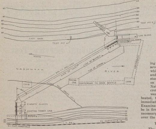
FIG. 2-LAYOUT OF DAM AND RELATED WORKS Test Pit A carried down to elevation 6.5 showed large boulders in impervious hardpan formation. No indication of rock. Digging discontinued at this elevation. Test Pit B carried down to elevation 3.5 gave results similar to those for Pit A.
