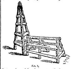
the top and spread three feet aps t at the bottom ; the whole being kept steady by reans of cross pieces of wood nailed upon them at regular intervals. Where the stack is built on an elevated frame, the appliance just described is placed in the centre, and the air enters from underneath ; but where the stack is built on the ground. . . . customary to use one or i.s, about two feet high and long enough to reach to the outsnie of the stack, for the purpose of securing the free admission of air.
