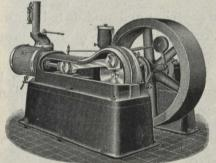
are all fitted with automatic governors and run at regular speed, whether loaded or light.
