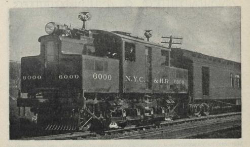
THE ELECTRIC LOCOMOTIVE BUILT FOR THE NEW YORK CENTRAL This style of locomotive will be used to draw the trains over the first thirty-five miles of their tracks running out of the Grand Central Depot, New York
