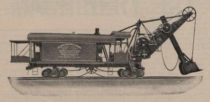
Direct wire rope hoist with but one sheave, instead of chain hoist with from five to seven sheaves, reduces delays and loss of time due to breakdowns, increases the efficiency of the engines, and reduces repair bills as well as fuel consumption.
