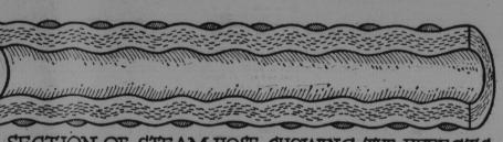
SECTION OF STEAM HOSE SHOWING THE EFFECTS OF WIRE-WINDING UNDER PRESSURE.
