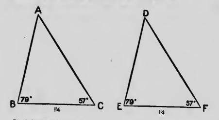
It follows, from 4, that the remaining angles at A and D are equal, each being 44°. Putting the points of the dividers on A and B, and carrying the dividers, so adjusted, to DE, compare the magnitudes of AB and DE. In like manner compare the magnitudes of AC and DF.
