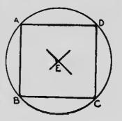
The lines from E to the angles are equal if the square has been accurately constructed and the diagonals accurately drawn; for the diagonals of all parallelograms bisect each other, and the diagonals of a square are equal.
