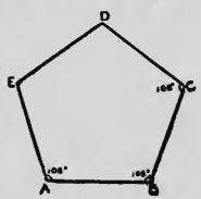
Joining E and D, we have a regular pentagon ABCDE. Using the bevel, we shall find that the angles at E and D are equal to the three other angles, and the dividers will prove the side DE to be equal to the other sides.
