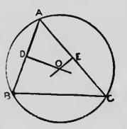
perpendicular to AB and AC, respectively. Then all points in DO are equally distant from A and B; and all points in EO are equally distant from A and C. Hence O is equally distant from A, B and C; and if the sharp point of the compasses be placed at O, and  $t^{\dagger}$  pencil end at A, or B, or C, and a circle be described, it will pass through A, B and C.
