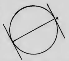
Evidently the tangents at opposite ends of a diameter arc parallel to one another.
