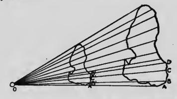
Suppose we wish to obtain a figure the same shape as ABC..., but with linear dimensions half those of ABC... Take a line OA'A, with OA' = A'A. From O draw a number of lines OA, OB, ... With the parallel rulers obtain B', through A'B' being parallel to AB; also C', through A'C' being parallel to AC;
