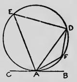
size between the angle CAD and the angle AFD in the alternate segment; and the relation between the angle BAD and the angle AED in the alternate segment.
