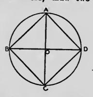
Of course the evident equality of the triangles AOB, BOC, ... proves the equality of the sides, and the angles ABC, BCD ... are all right angles, because they are angles in semicircles.
