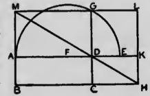
For, describe the square DGLK on DG, and let LK and BC meet in H. Then, if the figure has been accurately constructed, on producing the lines LG, HD and BA, they will be found to all pass through one point, M. Hence (Ch. VIII., 6) the square GDKL is equal to the rectangle ABCD.
