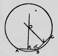
with which the angle ABC (135°) is constructed, AB and BC are bisected, and the perpendiculars KO and LO are drawn.
