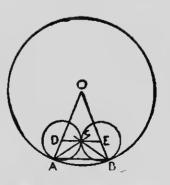
with D as centre, and DA or DC as radius, will touch the circle described with E as centre, and EB or EC as radius; and both circles will touch the large one.
