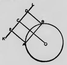
The chord AB is equal to ED, and therefore is of the required length, and it is parallel to KL.
