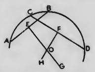
middle points draw perpendiculars EG and FH. The centre of the circle must lie on each of the lines EG and FH (Ch. X., 3), and therefore must be at O.
