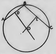
from the middle point of BC at right angles to it. Then all points in DO are equally distant from A and B; and all points in EO are equally distant from B and C. Hence O is equally distant from A, B and C; and placing the sharp point of the compasses at O and the pencil end at A, and describing a circle, it will pass through B and C, if the construction has been accurate.
