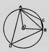
half of the marked angle AOB, is greater than one right angle. Similarly the angle ADB, being half the other angle at 0, is less than a right angle.
