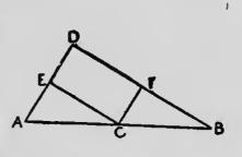
perpendiculars intersect in AB; and note also that C, being the centre of the circle through A, D and B, the centre of the hypotenuse of a right-angled triangle is equidistant from the three angles of the triangle.
