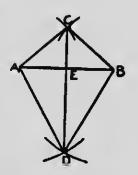
to the line CD—the figure on one side of this line being just the same as the figure on the other side, but turned in the opposite direction.
