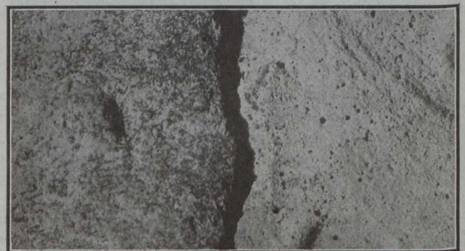
Fig. No. 30.—Surface Contact Between Under Side of Stone and Mortar Bed; 1:2½:5 Mix; First Consistency ( \times 5 )
