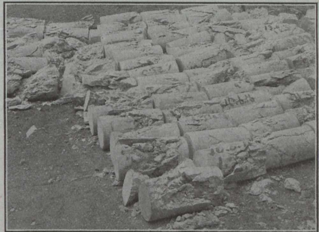
Fig. No. 19.—Broken Test Cylinders
