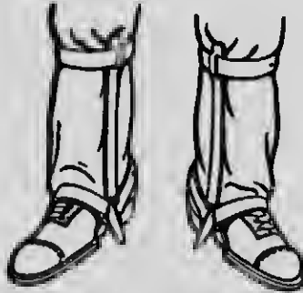
Fig. 28—Method of Attaching Pole Climbers to the Legs.
