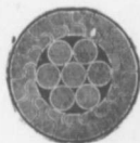
Locked Coil Aerial Cable or Colliery Guide.
