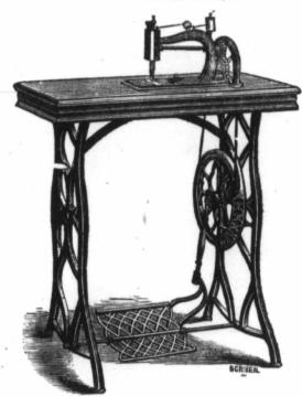
Represents Plain Family Machine, with solid shuttle and adjustable feed. The stand, has solid walnut table with drawer, brace, balance wheel guard, and well, working on hinges, in which the Machine is set—this well protects the clothes of the operator, and enables her to clean and oil the machine without changing her position, all of which makes it the most complete, simple, attractive and durable Family Machine in the market at the present time.
