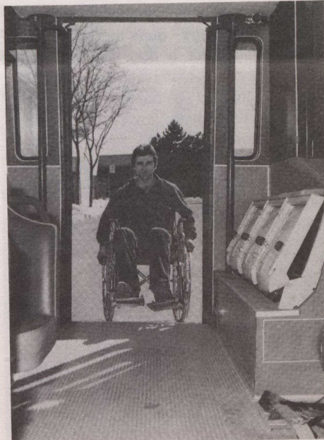
A "kneeling" system means the bus can be lowered for wheelchair passengers.
