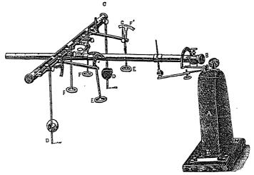
The object contemplated in the construction of this instrument, is to determine with exactitude the relation which exists between the volume of air which enters the lungs and the development of the body.
