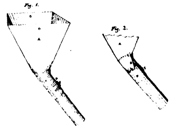
8535 Kirkby's Contrivance for Conducting Grain to the Eye of a Millstone.
