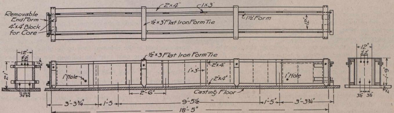
Plan, Elevations and Section of Concrete Girder Forms.
