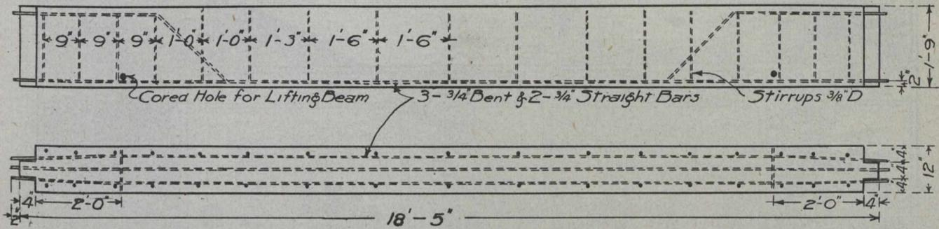
Plan and Elevation of Concrete Beam.
