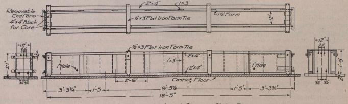
Plan, Elevations and Section of Concrete Girder Forms.
