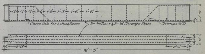
Plan and Elevation of Concrete Beam.
