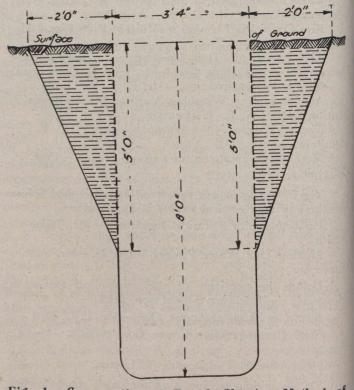
Fig. 1.—Cross-section of Trench Showing Method of Slicing in Sides in Caving Soil.
