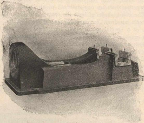
Fig. 7.—Medium-speed four-valve self-contained Frame.
