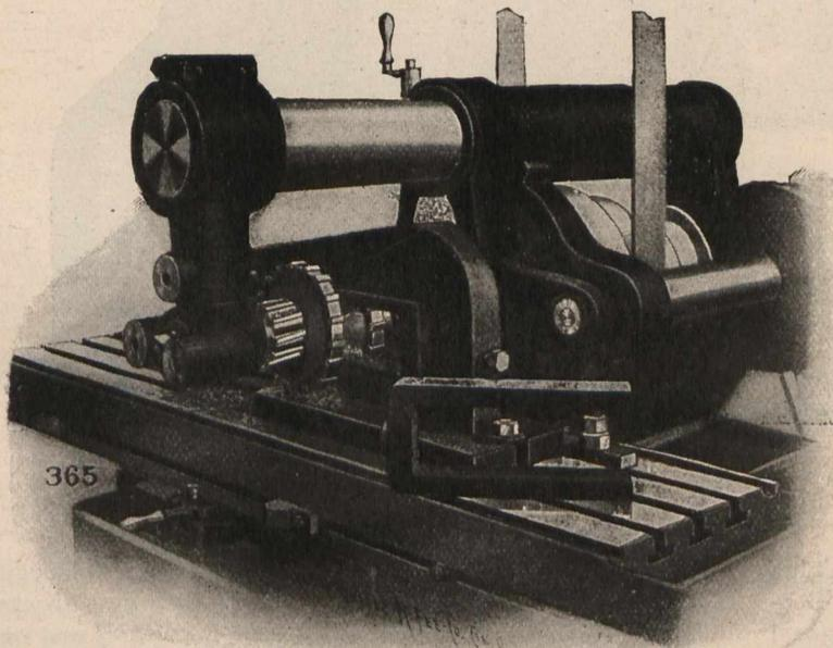
The first two operations shown in previous issues of "The Canadian Engineer," finished the ends and the sides of the straps. In this operation the two edges and the inside are finished. The piece is held in a convenient fixture, and the first cut taken is the one shown. In this the two side mills finish the edges of the piece, and a spiral mill between them roughs out the inside. The total width of
