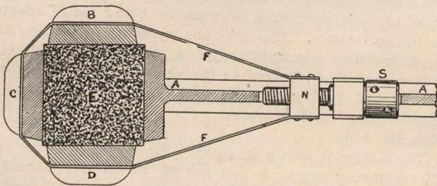
Fig. 26.—Electrode Holder of Heroult Steel Furnace.
