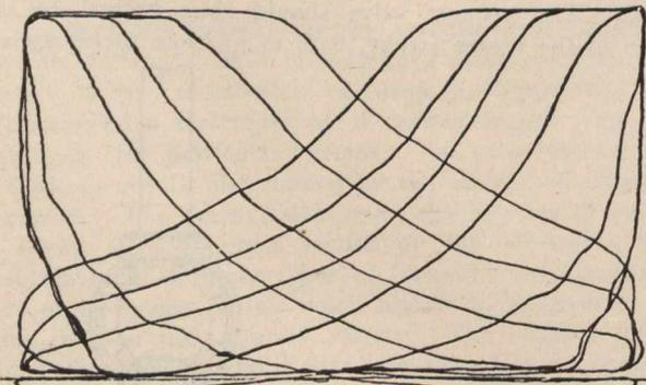
Fig. 4.—Indicator Card from four-valve engine.—
