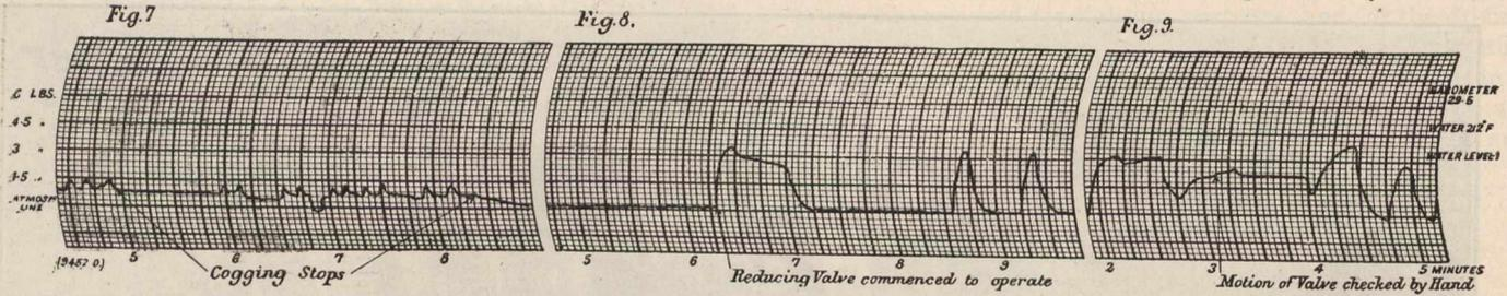
The regulation of the machine is excellent, and the speed variation of the turbine, when full load is thrown off, is not more than 5 per cent. momentarily, and the permanent variation, thanks to the Dennis compensator, is nil.
