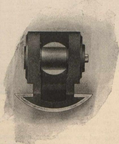
Fig. 10.—Cross-head of Medium-speed four-valve Engine.
