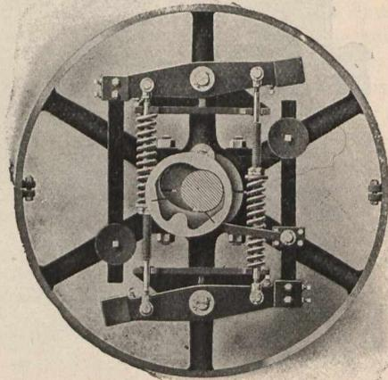
Fig. 5.—Atlas Automatic Shaft Governor four-valve centre crank type.
