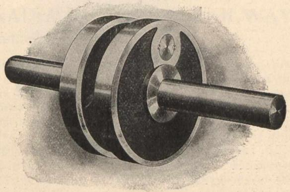
Fig. 9.—Four-valve Centre-crank Shaft.
