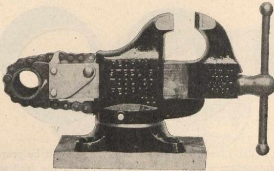
Fig. 3.—Long Single-swivel Vise with Pipe Attachment.
