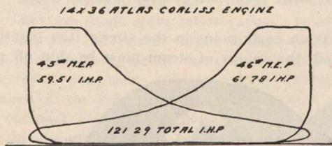
Fig. 3.—Indicator Card from Corliss Engine.—(96 R. P. M.)
