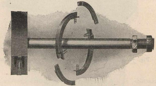
Fig. 12.—Piston and packing rings.
