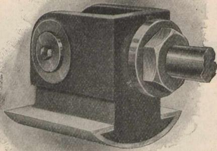
Fig. 11.—Cross-head of Medium-speed four-valve Engine. (three-quarter view).
