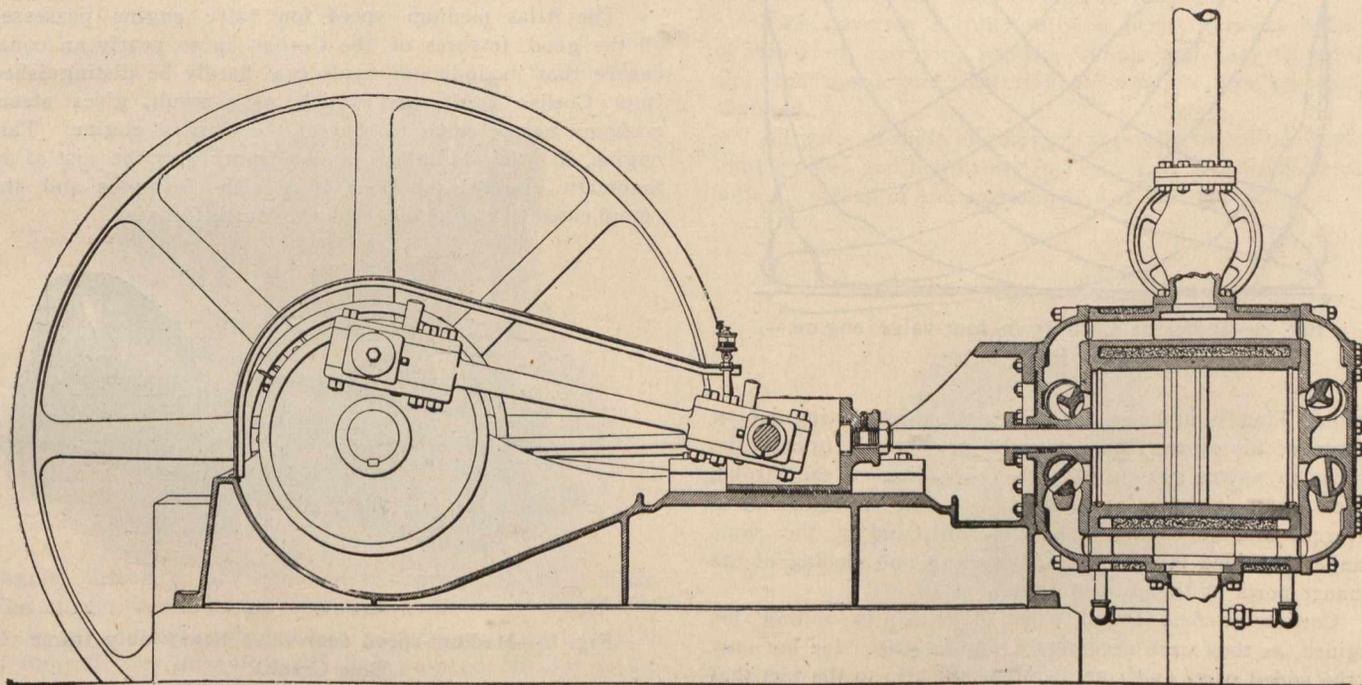
Fig. 2.—Automatic Four-Valve Engine.—Longitudinal Section.
