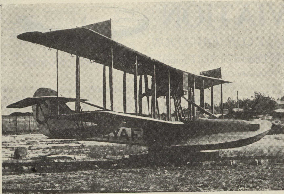
"H. S. 2 L" Flying Boat—1 Liberty Engine, 400 H.P., used at following air stations: Vancouver, Victoria Beach, Man., Sioux Lookout, Ont., Ottawa, Roberval, P.Q., and Halifax.
