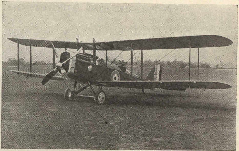
TYPE OF MACHINE USED BY THE AIR BOARD. "D.H. 4" Aeroplane—1 Rolls Royce Eagle VIII Engine, 360 H.P., used at High River Alta.
