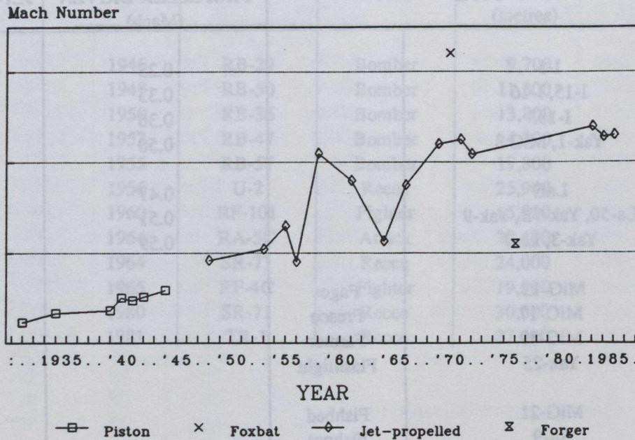
**Figure 20. Maximum Speed - Soviet Fighter Aircraft**
