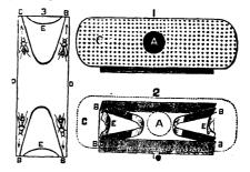
Fig. 2, shows the escape with the top removed. A is an outline of top entrance. B B B B are the outlets from the escape to the hive. C an outline of top plate; D D are side walls, and E E are circular end walls.
