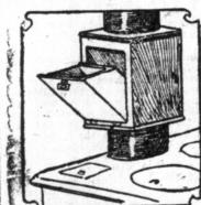
passage of the smoke, yet there is sufficient heat passing up the pipe to carbonize the solid garbage placed therein. The hopper is readily opened to deposit the waste, and when closed the odors pass up the chimney with the smoke. Whatever remains after the carbonizing process is readily emptied into the firebox, the hopper tilting downward for that purpose.
