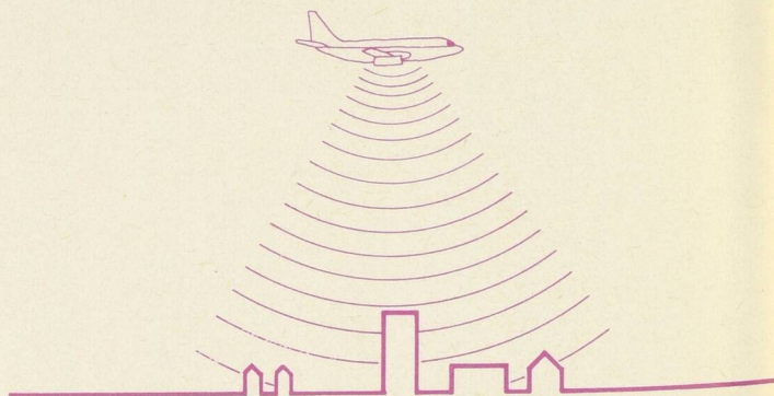
Flyover noise. As aircraft flies over, sound waves strike the house from a progression of different directions and distances.
