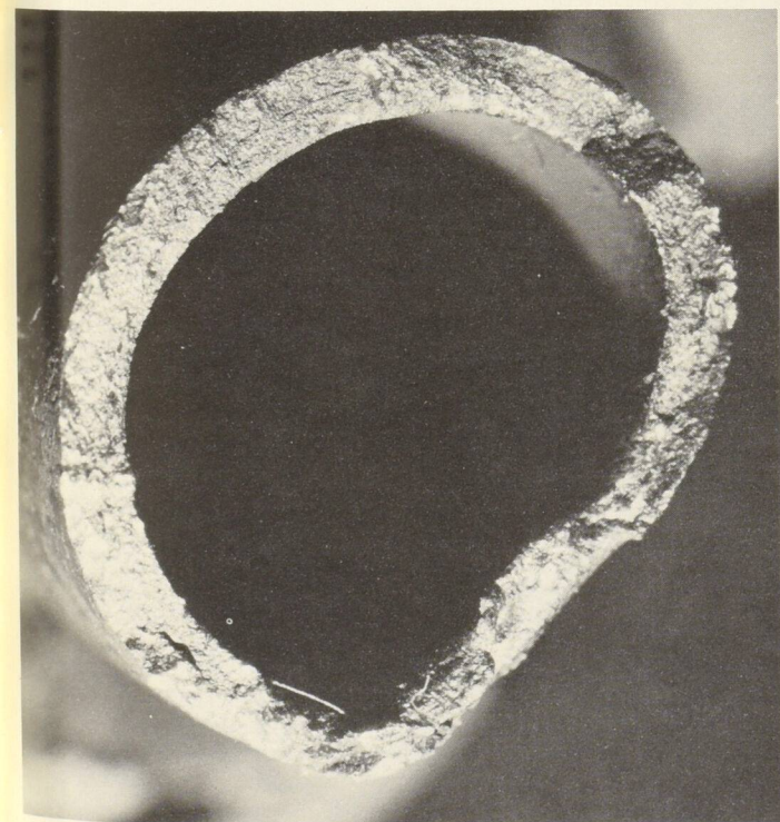
Fracture surface of the failed brake line tubing indicating the fatigue area and the rapid ductile fracture area. (Magnified 17 times).
