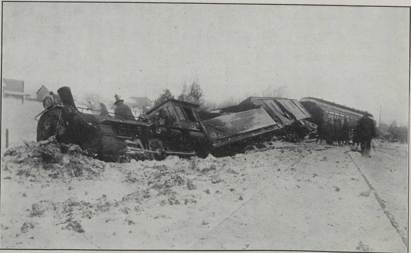
Accident at Hanover Passenger train No. 6, running between Owen Sound and Stratford was derailed about one and a half miles north of Hanover some days ago. The train was being hauled by two locomotives owing to heavy snow, and was travelling at the rate of about thirty miles an hour. The accident was caused by a steel plate about two feet by one having been fastened to the rail by some unknown person and was evidently a part of a land plough. The two engines and three first coaches were derailed, the engines being ditched, one of them completely turned round. Ten persons were injured.
