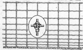
This fence is made in Canada enitrely of Canadian products. All the wires are full size true to gauge. Laterals and uprights are all No. 9 Hard Steel, well galvanized stock. Laterals are given a deep and continuous wave for "give and take." These coils or waves serve like a spring keeping the fence tight throughout all seasons and under all conditions. It is used by the principal farmers everywhere. The cost to you is no more than the price of other fence of equal weight. Insist on getting it.
