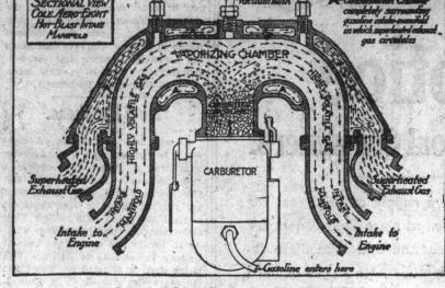
Operation of Aero-EIGHT Hot-Blast Manifold
