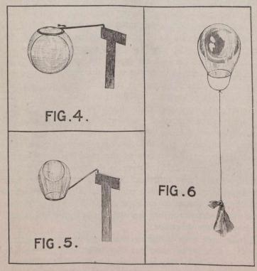
gas pipe, dipped first into the solution, is inserted through the bottom of the bubble about one-half inch. The gas is then turned on, and a gas bubble, as large as the original air bubble, blown and allowed to rest against the top of the external bubble. A gentle but firm downward jerk releases the pipe from both bubbles. This pull must be quick enough to prevent the meeting of the internal and external bubbles on the pipe, as this would result in their union.
