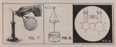
the extra weight required to produce equilibrium found. This gave the pull that the film exerted downward on the frame. In order to obviate as far as possible any error arising from the weight of the film, the frame should be wet for the first reading.
