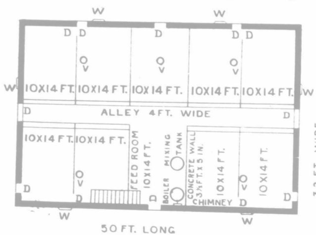
GROUND FLOOR OF PIGGERY BELONGING TO MR. ED. V. DECKER, ELGIN CO., ONT.
