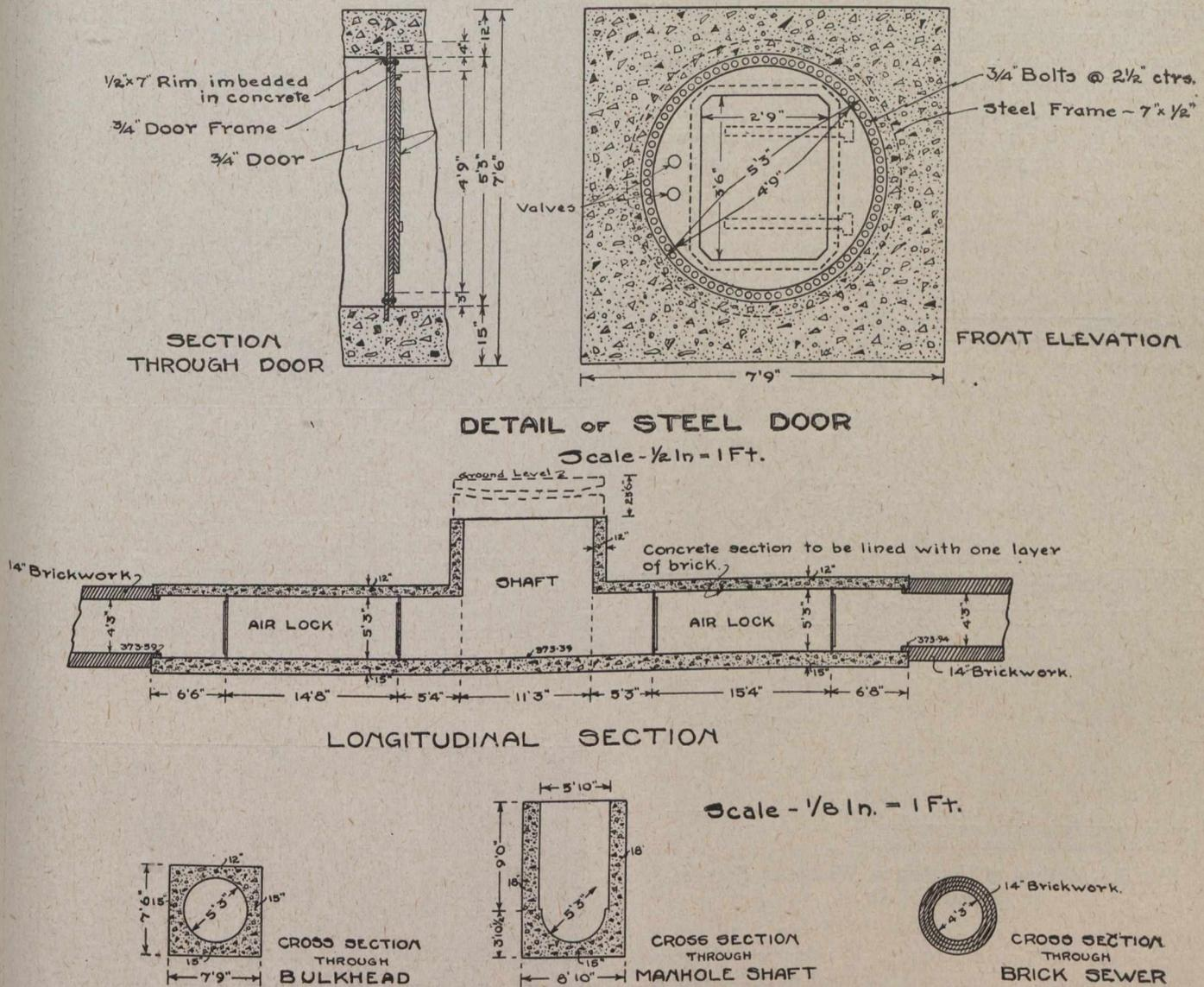
Fig. 3.—Details of Air Locks and Steel Door.
