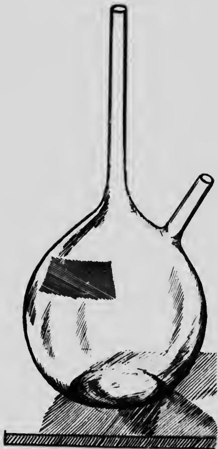
40. Viability flask of Jena glass. Capacity about 100 c. cm. The long neck may be sealed after growth is abundant. When it is desired to transplant, the tube may be cut off, and resealed in the flame. There is ample length to repeat this several times if necessary.
