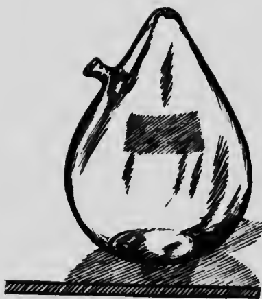
39. Viability flask of Jena glass. Capacity about 50 c. cm.
