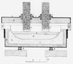
Fig. 23.—Heroult Steel Furnace.
