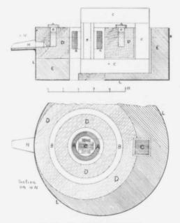
Fig. 24.—The Kjellin Steel Furnace.
