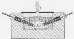
Fig. 4.-Cowles' Furnace for Aluminum Alloys.
