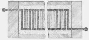
Fig. 41.-Multiple Core Furnace.
