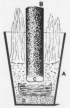
Fig. 7.—Willson's Carbide Furnace. more coke to form a carbide. These reactions may be represented by the following chemical equations, which also indicate the relative amounts of lime and coke to use in the charge :—
