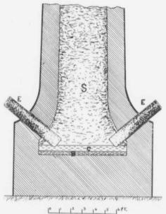
Fig. 31.—The Harmet Furnace.
