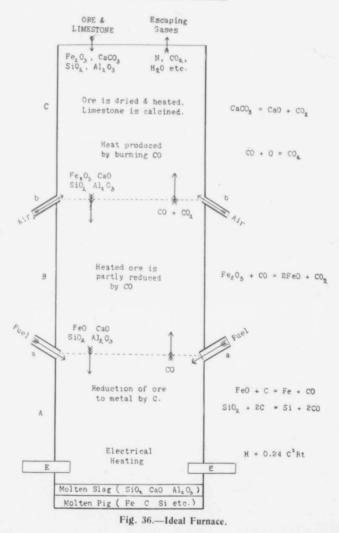
the fact that no use was made of the escaping furnace gases. It is very desirable to know what improvement in efficiency may be expected when all possible improvements have been made in the design and construction of the electric smelting furnace, and what is the minimum amount of fuel and electrical energy that will then be needed. For this purpose the operation of an ideal furnace may be studied, omitting for the present any consideration of how such a furnace could actually be constructed.
