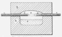
Fig. 10.-Independent Arc Furnace.
