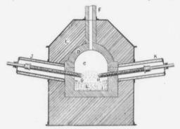
Fig. 37.-Stassano Furnace.
