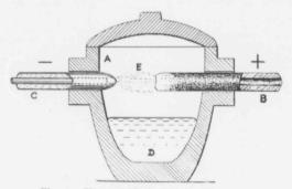
Fig. 3.-Siemens' Horizontal Arc Furnace.
