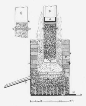
Fig. 29.—Heroult Ore-smelting Furnace.
