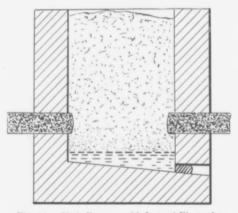
Fig. 16.—Shaft Furnace with Lateral Electrodes.
