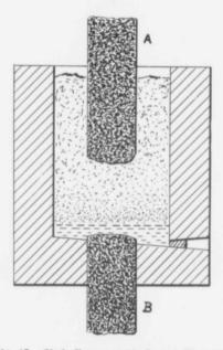
Fig. 17.-Shaft Furnace with Central Electrode.
