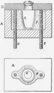
Fig. 13.-Electric Crucible Furnace.
