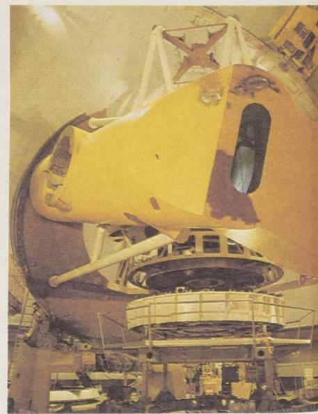
The eye of the telescope, its 3.66 m primary mirror, looks up from the circular support "cell" below the yellow beams. Whether used horizontally or at different angles, the mirror lies on a bed of pressurized air pads which keeps it from distorting under its own weight. The same Canadian-designed system was used in Victoria to cushion the mirror during the grinding and polishing operations. (Photo: W.J. Cherwinski)
