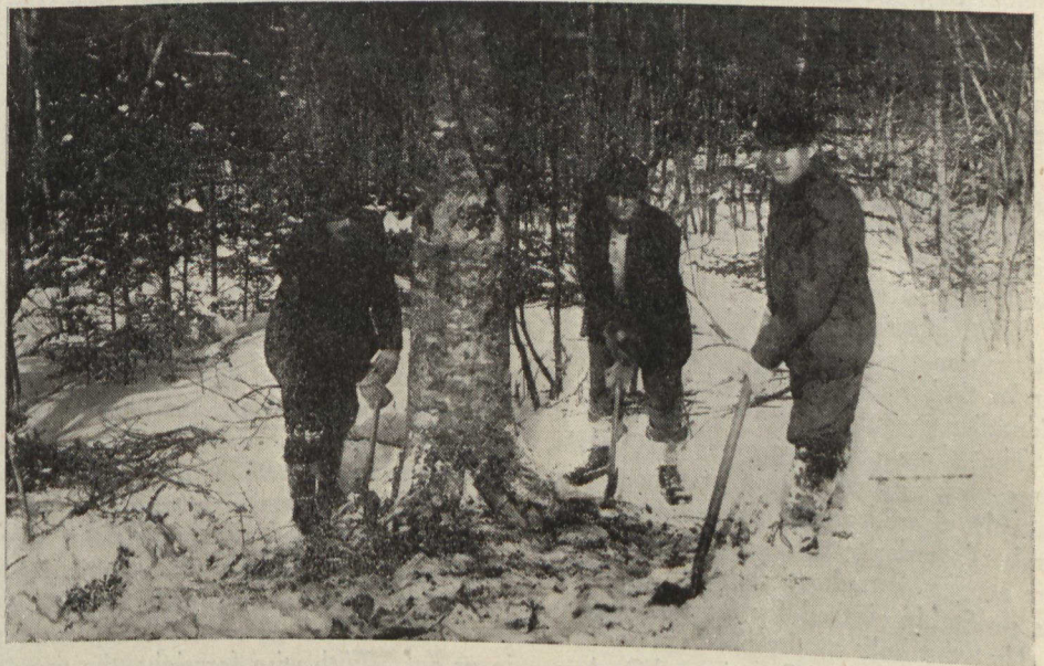
MAKING "SHIP KNEES" FOR NOVA SCOTIA'S WOODEN SHIPS. A scene in Yarmouth County where the axemen are carefully felling a tree, taking a portion of the curved root which forms the bow of the boat.
