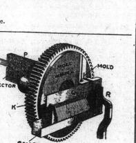
FIGURE 2. Mold wheel in position for casting a line.
