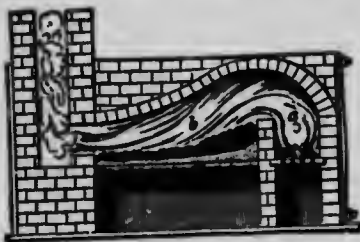
Section of Reverberatory Furnace.
