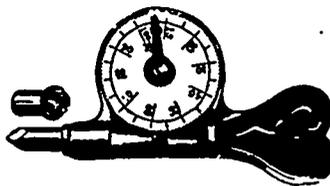
combine to make this indicator, its makers claim, preferable to any other in use. It is adapted to pointed or hollow centers and has a raised sight on dial so as to count by touch, which is of great importance, especially in dark places, as it is only necessary to look at your watch and count the number of revolutions the dial makes, which, with the fractions, will be the exact speed
