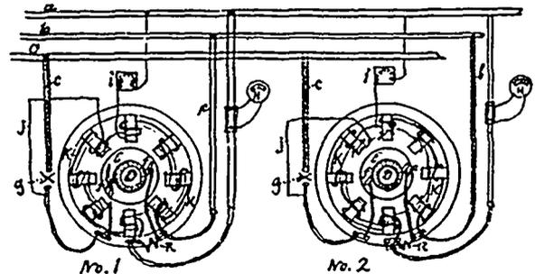
a. Positive bus bar. b. Equalizing bar. c. Negative bar. d. Commutators. e. Armatures. f. Brushes. g. Circuit breaker. h. Ammeter. i. Rheostat. j. Shunt field. k. Series field. r. German silver resistance.
