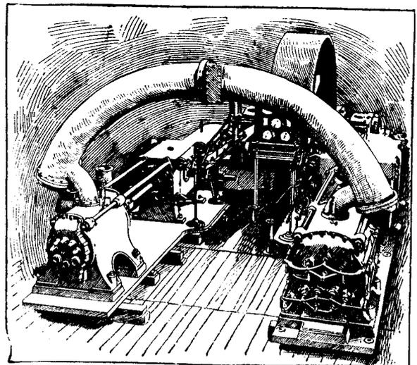
a fly-wheel 16 feet in diameter, 40 inches face, weighing about 28,000 lbs., which insures the steady running of the machine. The machine weighs about 240,000 lbs., and was shipped in six car loads to the Le Roi Mining Co., at Rossland, B.C.
