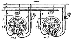
a. Positive bus bar. b. Equalizing bar. c. Negative bar. d. Commutators. c. Armatures. f. Brushes. g. Circuit breaker. h. Ammeter. i. Rheostat. j. Shunt field. k. Series field. r. German silver resistance.
