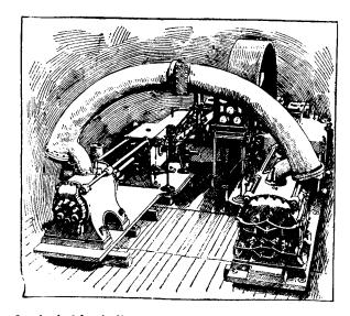
a fly-wheel 16 feet in diameter, 40 inches face, weighing about 28,000 lbs., which insures the steady running of the machine. The machine weighs about 240,000 lbs., and was shipped in six car loads to the Le Roi Mining Co., at Rossland. B.C.
