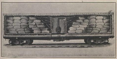
Fig. 1. Warm air circulation in correctly lined and loaded car of potatoes.
