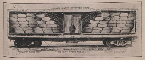
Fig. 2. Warm air circulation in an incorrectly lined and loaded car of potatoes. The warm air from the stove cannot reach space beneath the false floor, where it is needed.
