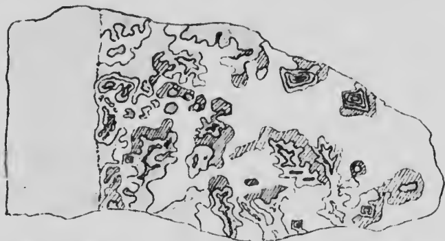
Fig. 30. Diagram of portion of vein from Silver Bar mine, natural size, showing order of deposition. The shaded part represents smaltite-chloanthite intergrowth with chloanthite in the centre of dendritic growths. The hatched part is later niccolite and the white is eudrite.
