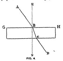
A ray of light, EB, from the air incident to a sheet of glass, GH, passes through the latter in a straight line.
