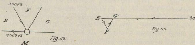
notice that the Vector Polygon reads ME, EF, FG, and GM. This last line GM coincides with the first line ME, the sense mark of ME having been placed above and that of GM below.)
