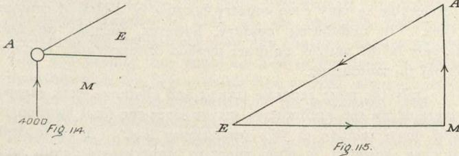
against the point and the force EM away from the point. The magnitudes of the forces AE and EM will be given by scaling AE and EM (Fig. 115). The member AE is, therefore, in Compression and the member EM in Tension.
