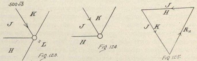
structing the Vector Polygon for this last set of forces, it is seen from Fig. 125 that HJ acts away from the point, thereby showing that the member HJ is in Tension.
