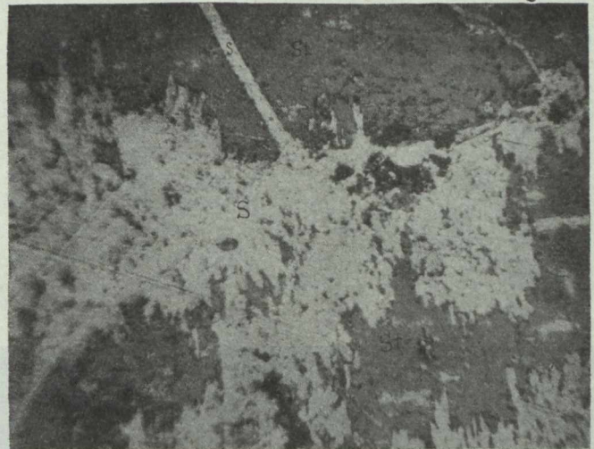
PLATE IV Stephanite (St.) replaced by veinlets and desiminations of silver (S). Mag. 300 diameters.
